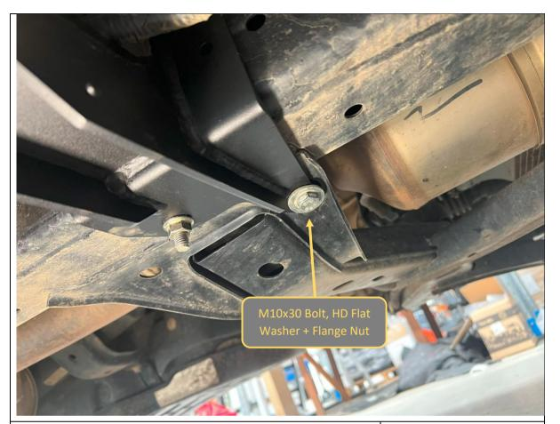
17. Once secure, finish front mount installation securing final mounting point with M10x30 Bolt, HD Flat Washer, and Flange Nut.
