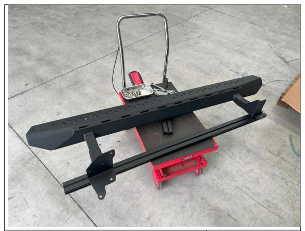
13. Unpack welded slider assembly and position on lifting trolley such that mounts sit approximately level.
